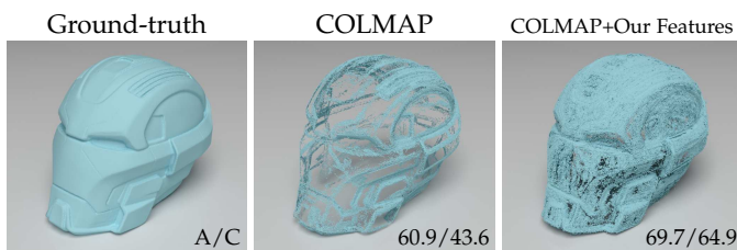
Fig. 14: Boosting another MVS method (COLMAP) with our features. From the left to right: the ground-truth, geometric reconstruction by COLMAP from environment-lit images, and the result by sending our feature maps to COLMAP. Quantitative errors in accuracy/completeness percentage are indicated in the bottom right corner.
